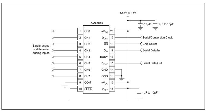
FIGURE 1. Basic Operation of the ADS7844.
