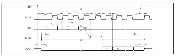
FIGURE 5. Detailed Timing Diagram.
