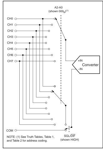
FIGURE 2. Simplified Diagram of the Analog Input.
