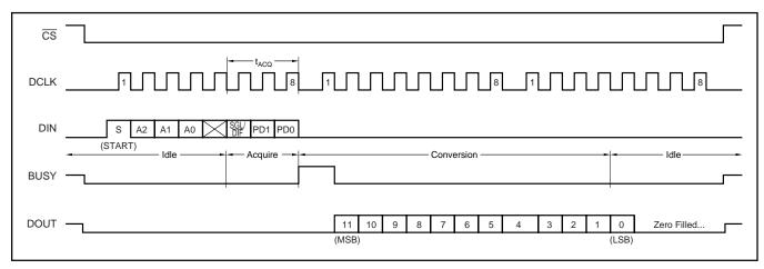
FIGURE 3. Conversion Timing, 24-Clocks per Conversion, 8-Bit Bus Interface. No DCLK delay required with dedicated serial port.
