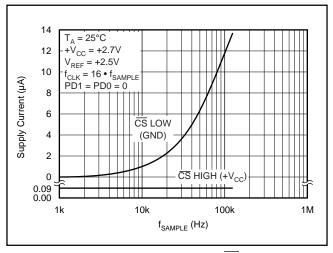
FIGURE 9. Supply Current vs State of  $\overline{CS}$ .
